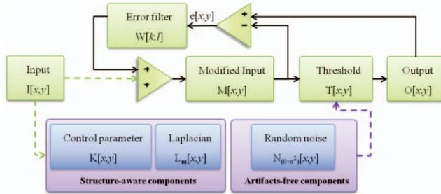
**Figure 1. Block diagram of the proposed error diffusion algorithm.**
