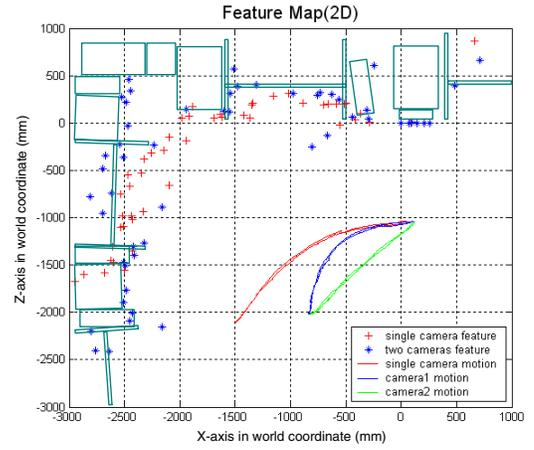
Fig. 11. The final 2D map of camera motions and features on XZ-plane. In the same camera, the camera motion is more accurate in one of the two cameras(blue) compared with a single camera(red).
