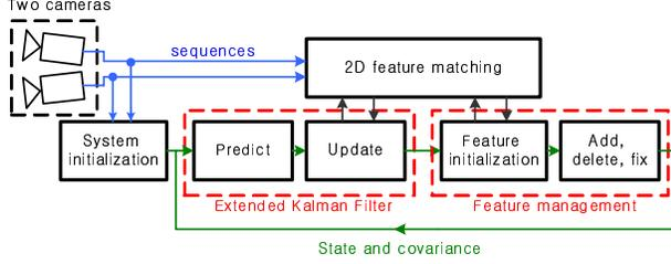
Fig. 1. The overall flow of the system.
